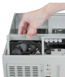
Easy-to-maintain cooling fan
